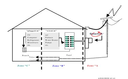
If your home experiences a high voltage surge without whole house surge protection, wired appliances/equipment within Zone B will not be protected and outlet plug-in strips provide limited protection, if any, for plugged-in appliances within Zone C.
